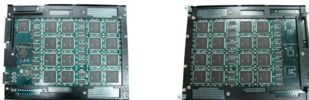
**Figure 1.** Front and back sides of the board of the RCS MPA basic module
